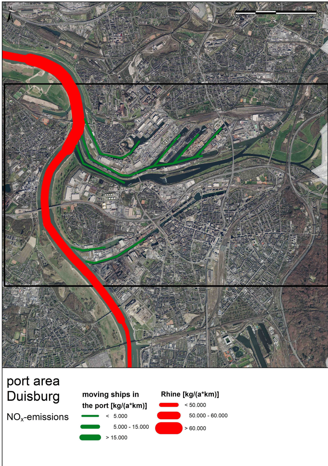
Figure 4: NO x emission densities of the moving ships in the Duisburg study area Inner box: Boundary of the port area
